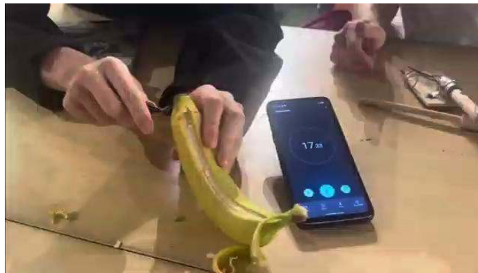
Figure 2.2.2: Clip from video using rolling motion to peel banana. This was a proxy device as the geometric prototype was unable to complete the motion.
